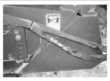
12. Remove the union fitting from the two-piece lead hose.
