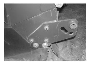
1. Attach the mount plate with the three carriage bolts and lock nuts provided.
