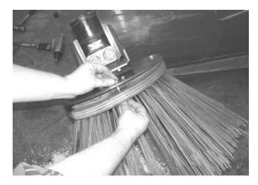
6. Mount the hub plate to the motor using the woodruff key and nut.
