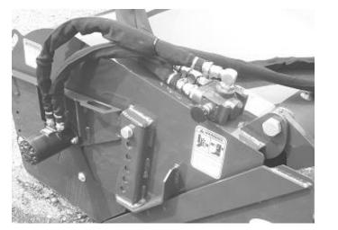
13. Connect the shorter hose from the motor to the elbow fitting on top of the selector valve. Connect the longer hose to the tee fitting.
