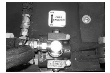
14. Clean the surface of the hood next to the valve block, and install the "On-Off" decal as shown.
