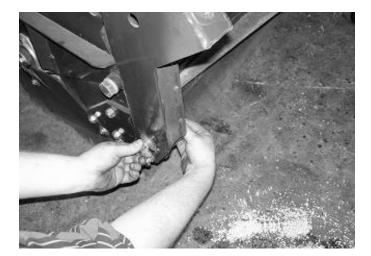
2. Mount the sweeper arm to the mounting bracket using the 3/4" x 3-1/2" bolt and lock nut provided. Position the sweeper arm in the up position, and secure in place with the 3-point pin and lynch pin.
